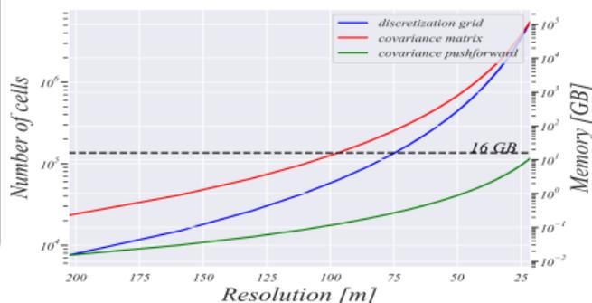
Figure: Grid and matrices size vs resolution on Stromboli example.
